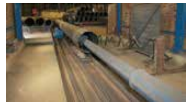
Full length radiographic inspection
