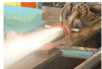
Hydrostatic testing and ultrasonic inspection
