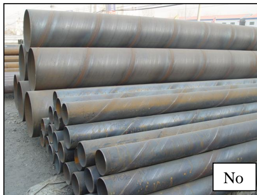
Figure 4: Spirally welded pipe – not a cast iron pipe
