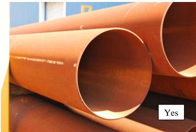
Figure 3: Longitudinally Welded pipe that is internally scarfed
