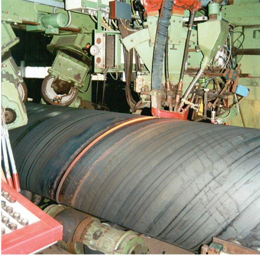
E2. External welding
