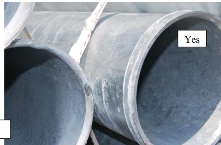
Figure 2: Welded pipe externally scarfed and internally scarfed
