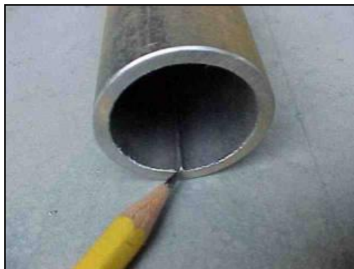
Figure 2.7 Tube produced by the HFI ERW method with the linear weld bead clearly visible on inside weld seam
