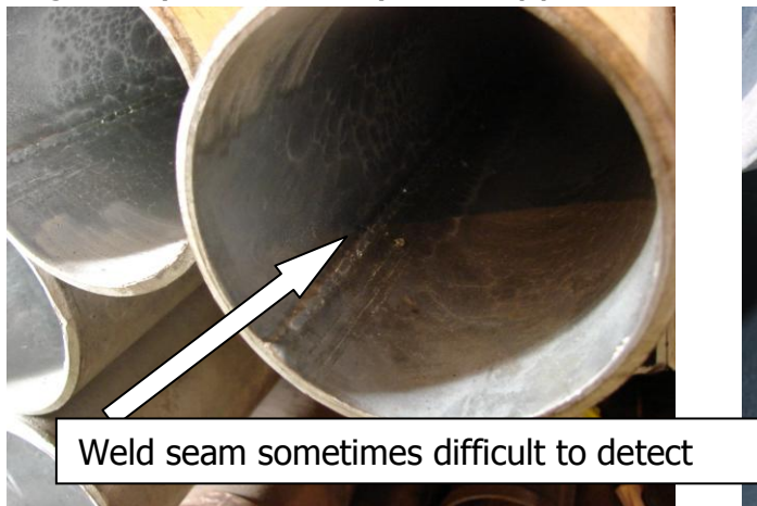
Figure 1 : Longitudinally welded, internally unscarfed pipe
