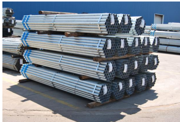
Figure 5: Internally scarfed galvanized tube
