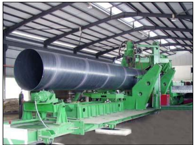
Figure 2.12 Spiral pipe mill (a) strip entry and (b) mill exit
