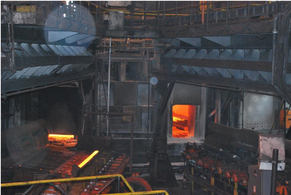
B4. Rotary furnace with billets inside
