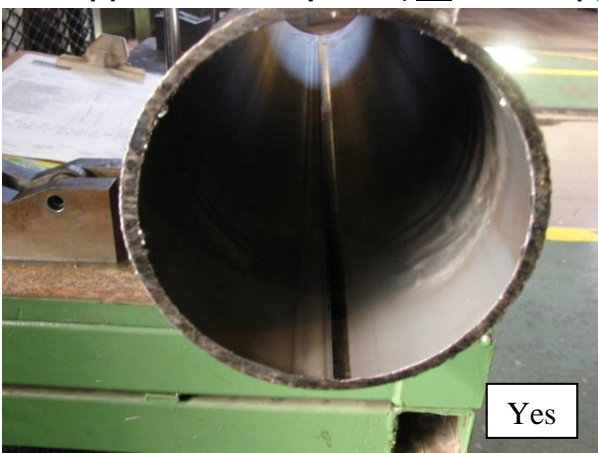
Figure 3: Welded pipe that is internally scarfed, not a cast iron pipe
