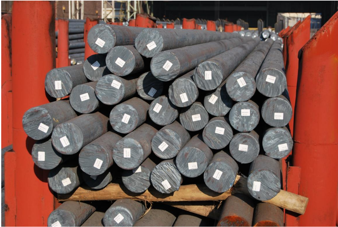
B3. Steel billets before seamless pipe mill
