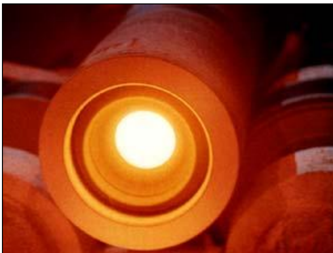
Figure 4.2 Cast (Ductile) Iron Pipe being (a) cast in a spinning mould and (b) withdrawn from the mould
