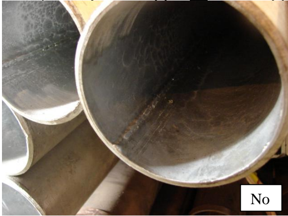
Figure 3: Welded pipe that is internally scarfed, not a seamless pipe
