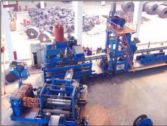
Figure 2.12 Spiral pipe mill (a) strip entry and (b) mill exit
