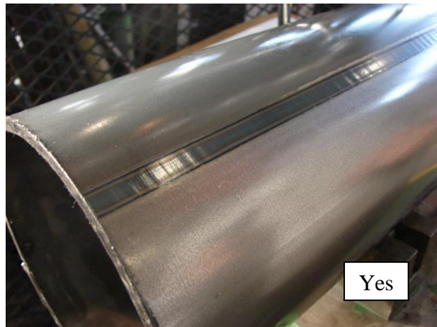
Figure 4: Spirally welded pipe – not a cast iron pipe
