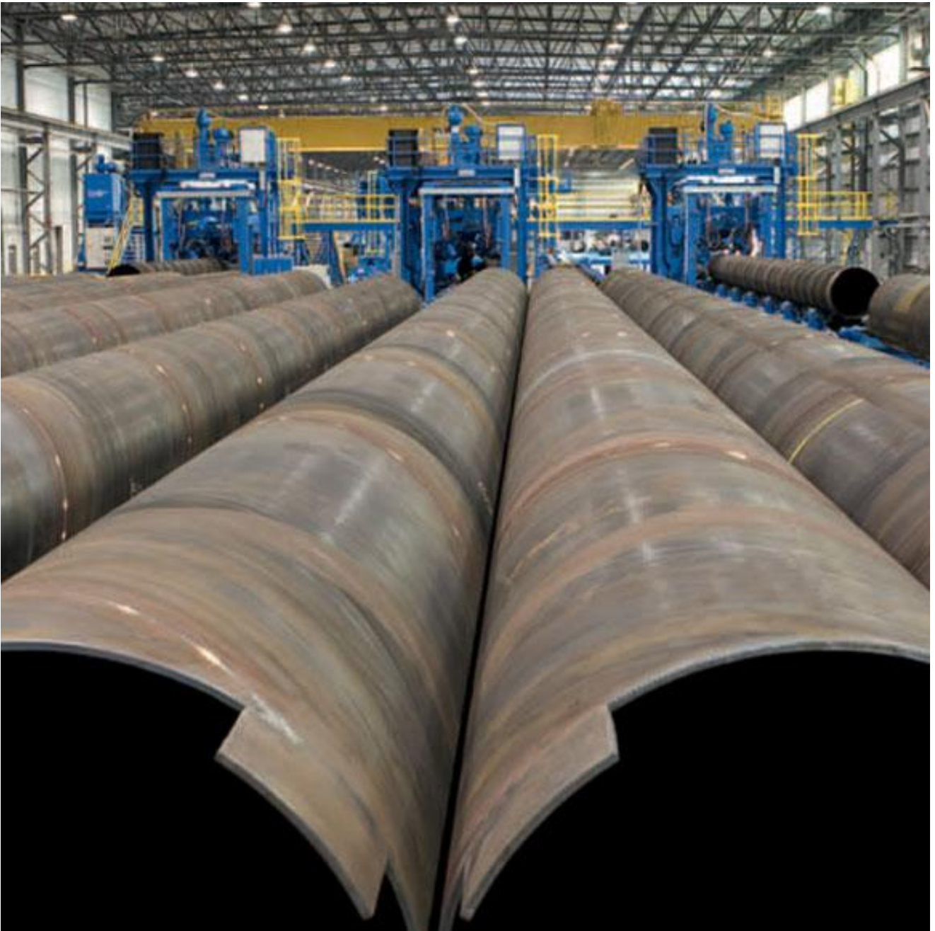
E3. Spiral pipe after welding
