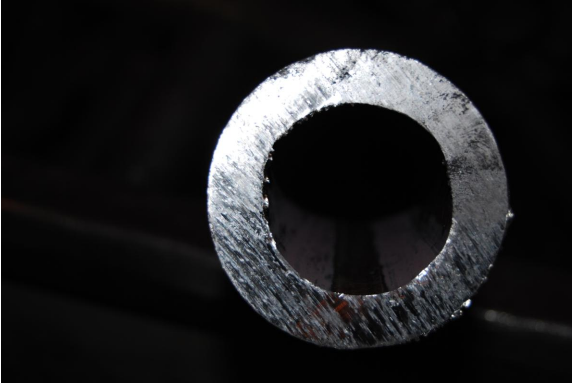
B7. Seamless pipe end before bevelling
