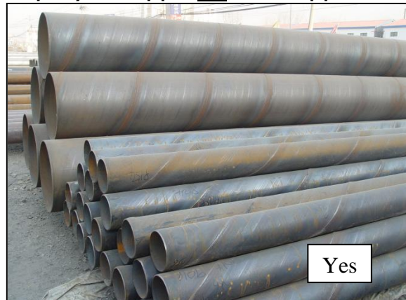
Figure 4: Spirally welded pipe – not a cast iron pipe
