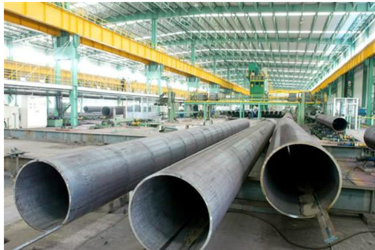
Figure 2.10 LSAW Pipe with weld seam visible at the bottom. Note welding tabs still attached to pipe end.
