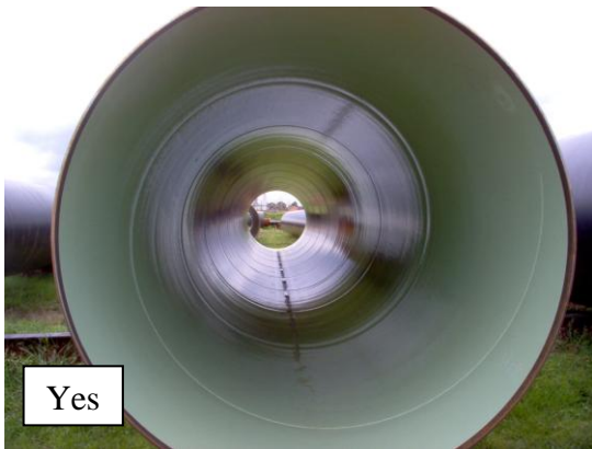
Figure 3: Longitudinally Welded pipe that is internally scarfed
