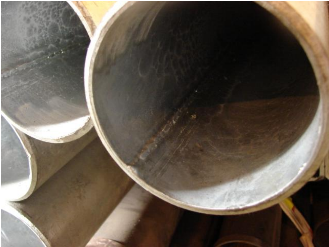
C5. Inside weld bead not removed (unscarfed)
