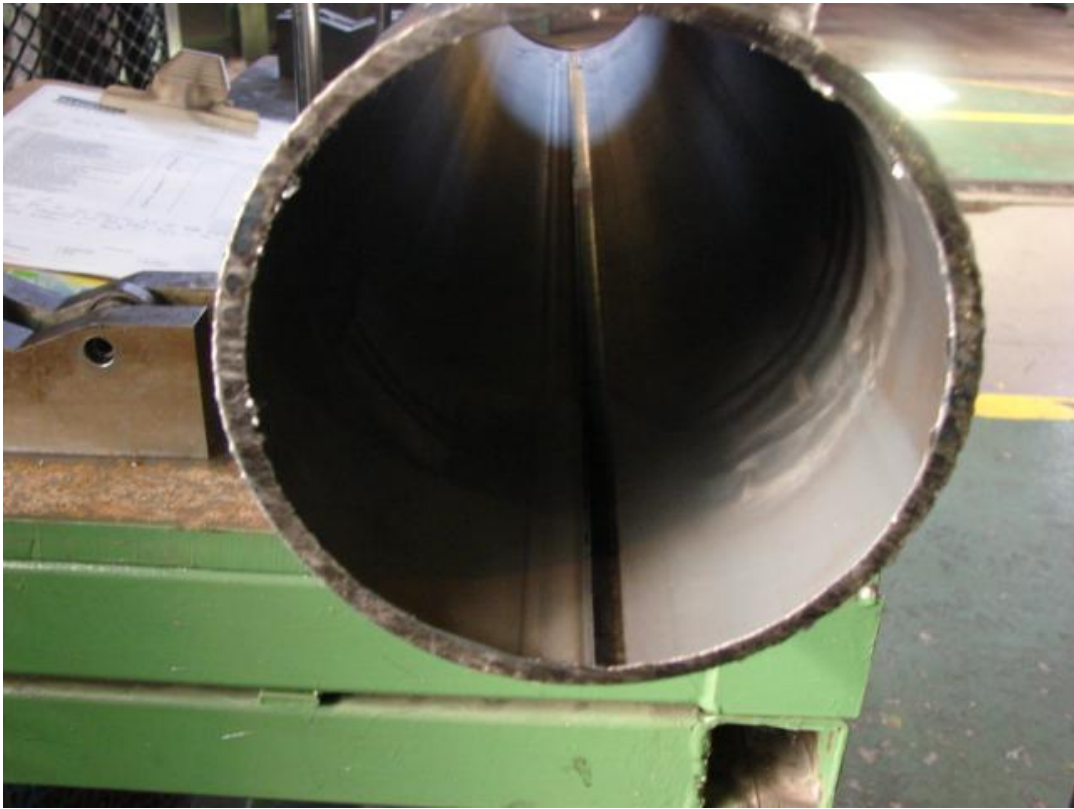
C4. Inside weld bead removed (internally scarfed)
