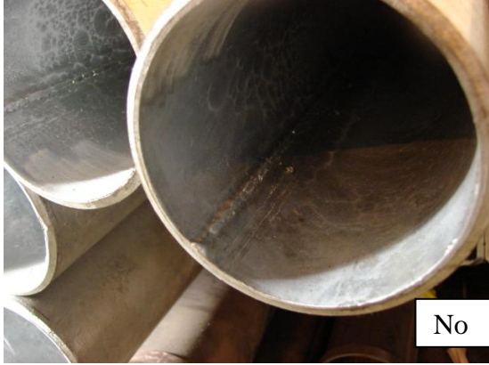
Figure 1 : Welded, internally unscarfed pipe – not a seamless pipe
