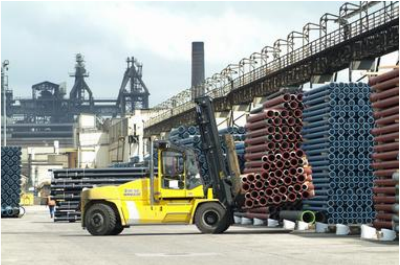
A.1 Handling the ductile cast iron pipes in the factory yard
