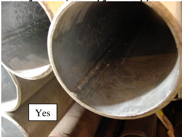
Figure 3: Welded Galvanized Pipe
