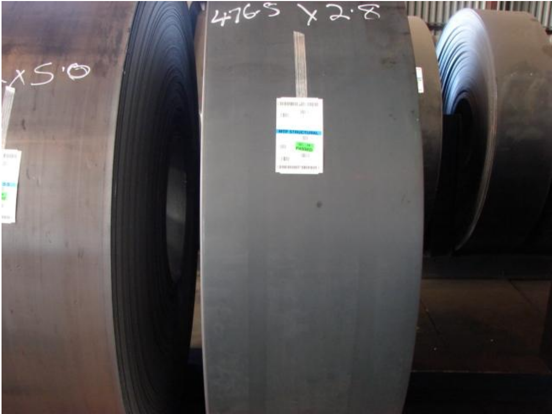
C2. Slit mults ready before ERW tube mill
