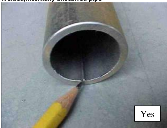
Figure 1 : Welded, internally unscarfed pipe
