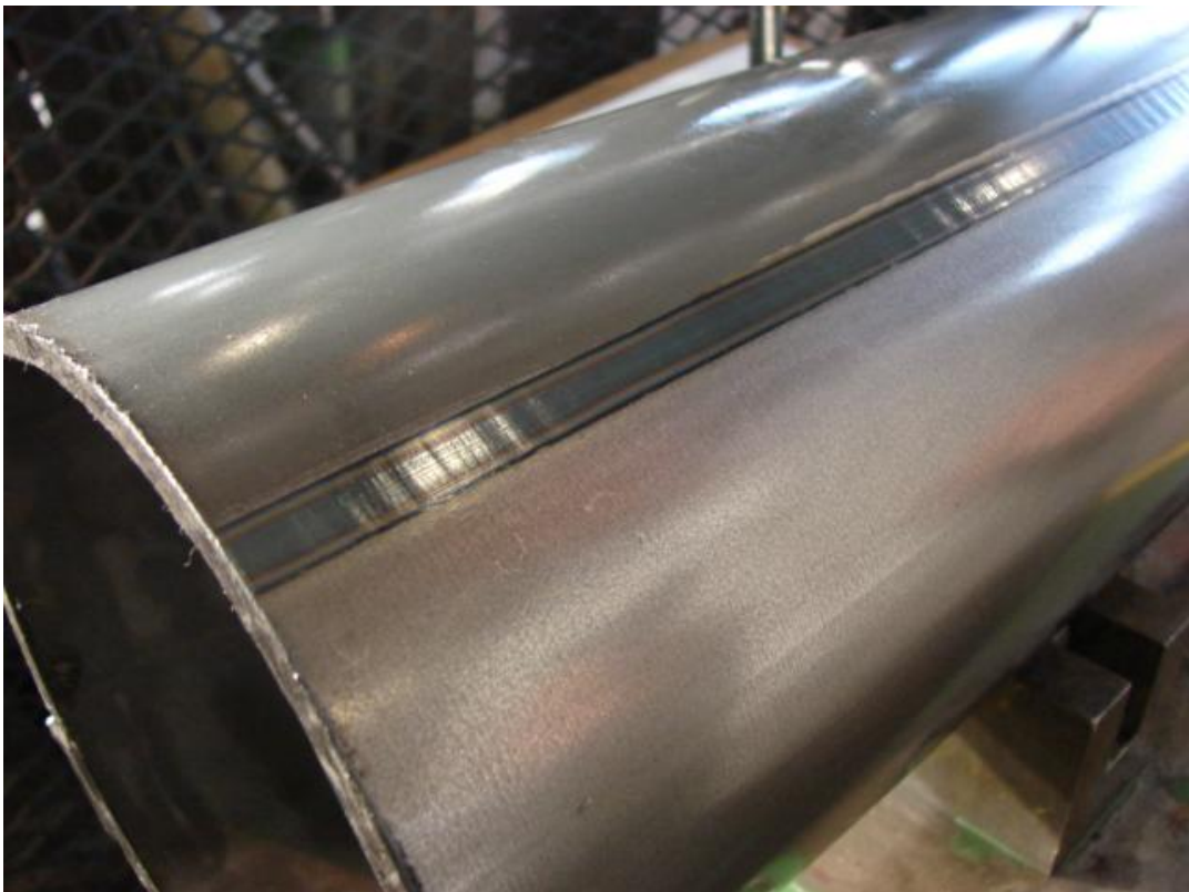
C3. Externally scarfed weld seam on round tube
