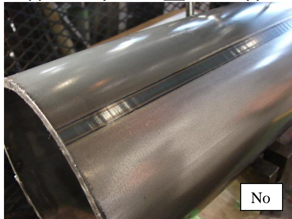
Figure 4: Spirally welded pipe – not a seamless pipe
